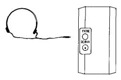
Because the radio can receive stereo FM, when you listen to FM stereo broadcasts, be sure your headphones are designed for stereo operation so that you can obtain the full benefit of this feature.
